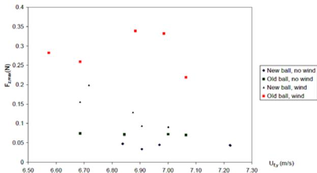
Figure 7. Lateral force versus fall velocity of a new and a used cricket ball with and without the wind tunnel operating.
