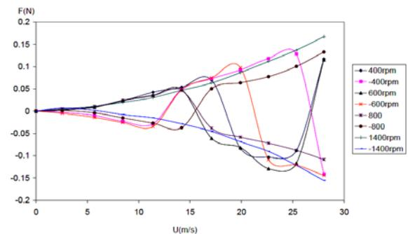
Figure 5. Lift force versus free stream velocity for ball No.4.
