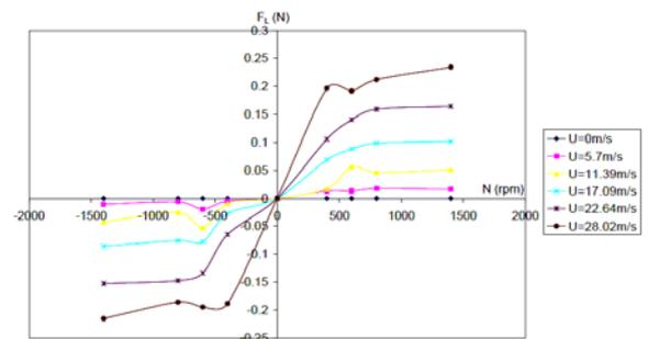
Figure 4. Variation of lift force with rotation rate of the ball No.1.
