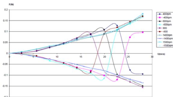
Figure 6. Lift force versus free stream velocity for wooden ball No.W1.
