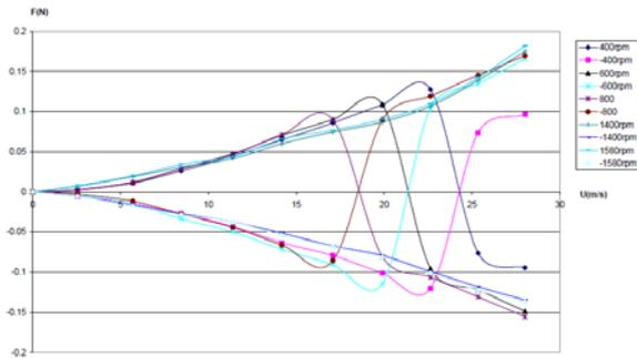
Figure 6. Lift force versus free stream velocity for wooden ball No.W1.
